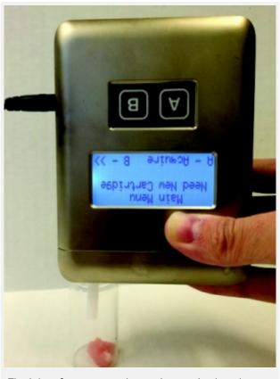
The inlet of a compact electronic nose is placed near a meat sample to detect freshness.
